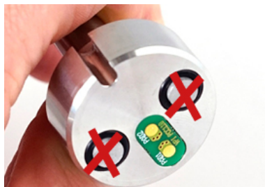
1a. Remove sinter filter. Do not re-use!
